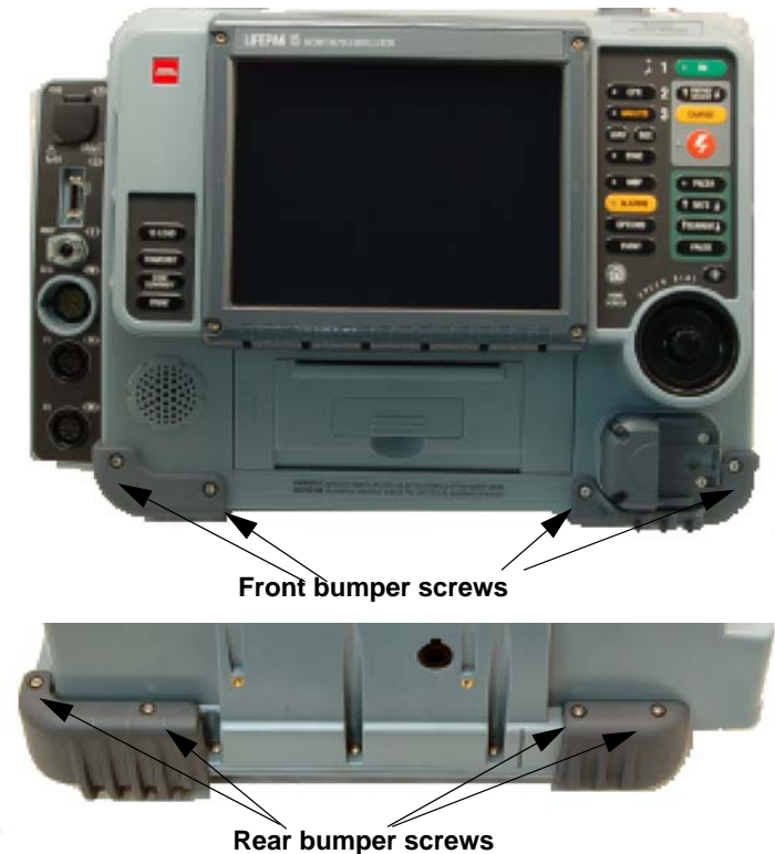
Figure 8.3—Bumper screw locations
