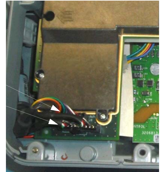
Figure 8.41—ECG and IP/Temp connections
