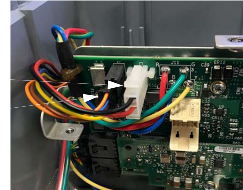
Figure 8.55—Power PCB connections (REF 21330-001555 )
