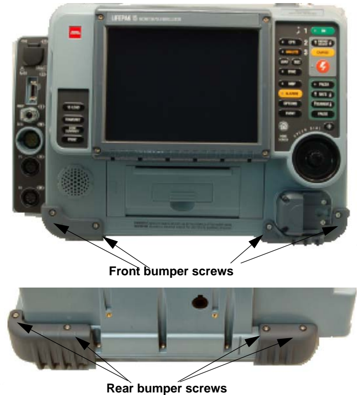
Figure 8.8—Bumper screw locations
