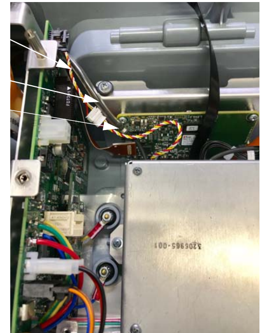
Figure 8.75—CO2 module connections
